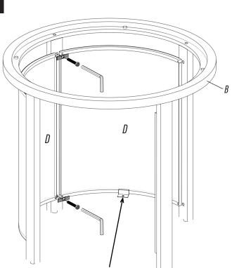
When installing part "D", Please note that the side with this part is facing down.
