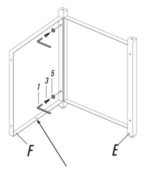
When installing part "F", Please note that the side with the hole is facing down.
